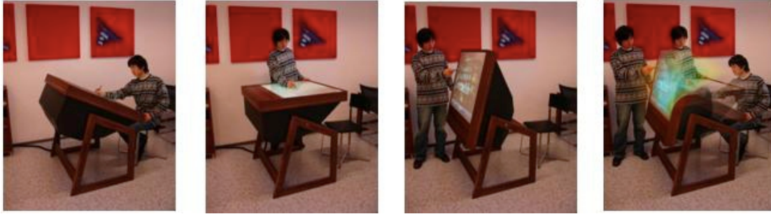
Figure 15. FLUX Multi-touch and Pen Support with tilt adaptation
