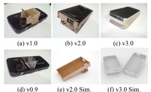
Figure 4. Development stages of the phone case prototype. (e,g) 3D rendering of the prototypes design.
