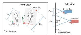
Figure 3. Rectification of the characters using the projected markers, under the assumption that the projectors and cameras are positioned perpendicular to the projection plane. The relation between  $d_{RED}$  and  $d_{BLUE}$  and the angle  $\theta$ , determine the rigid transformation applied to the red character.
