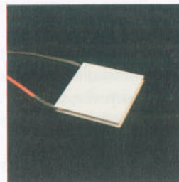
▲ Figure 4-20 In a Peltier device an input electrical current causes one face to heat up and the other to cool down. Ceramic plates are used in the device shown. It is necessary to transfer heat away from the hot surface via fans or heat spreaders. Peltier devices are used in many products, including drink coolers and in computers to cool microchips
